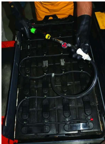
Figure: Technician using a single-point watering hose with flow indicator (red “X” device) to fill all cells of a forklift battery safely and evenly.
